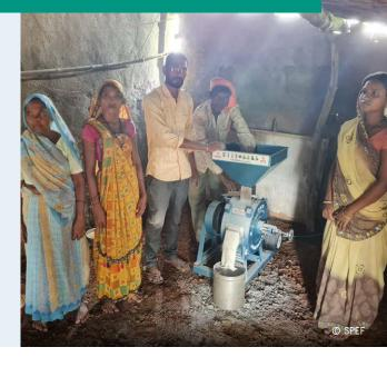
which also significantly cuts down the travel costs leading to community savings as farmers had to travel long distances for milling of their produce.<sup>29</sup> An off grid solar power grain grinder provides a relatively stable power source. Using a diesel generator is not the best option given the increasing fuel prices and diesel is not easy to access in many rural areas.
